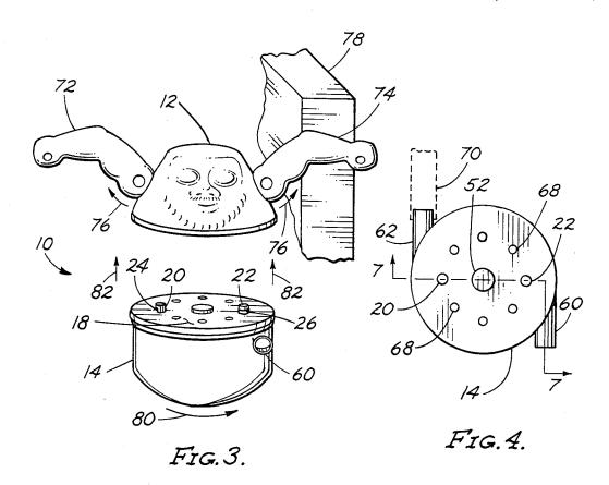
Figure 2. Toy Top with Impeller-Driven Flywheel, U.S. Patent No. 4,772,241 (filed July 22, 1987) (issued Sept. 20, 1988).
